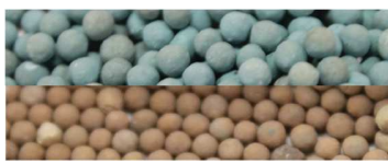
Moisture Adsorbent: Top: Full Capacity; Bottom: Depleted.
