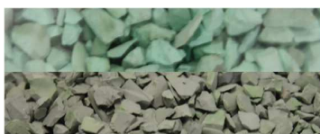
Oxygen Adsorbent: Top: Full Capacity; Bottom: Depleted.
