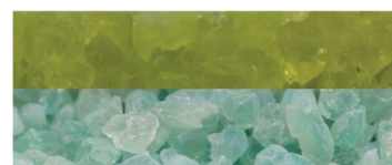
Co Free™ Adsorbent: Top: Full Capacity; Bottom: Depleted.
